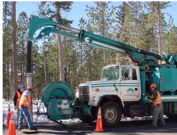
The City's jet/vacuum truck is used on emergencies and routine sewer cleaning. Frequent cleaning of trouble spots resulted in zero overflows, zero sewage spills and zero damaging backups in 2006.
